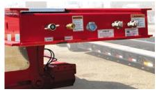
Simple, quick and easy hookups to any tractor air, electrical and hydraulic system.
