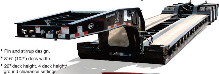
Hydraulically operated by PTO/wet line or optional power pack.
