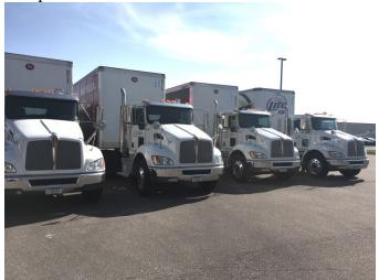
The Kenworth T370s put into service – 25 in Florida, and 18 in Minnesota – are powered by the PACCAR PX-9 engine rated at 300 hp, and use Allison automatics. "We haul 28- and 36-foot rear loading trailers with our T370, which can accommodate up to 700 cases on the smaller trailer and up to 1,200 cases on the 36-footer," said Rivera. "To give us flexibility, and different hauling capacities, we have both single and tandem axle T370s."
