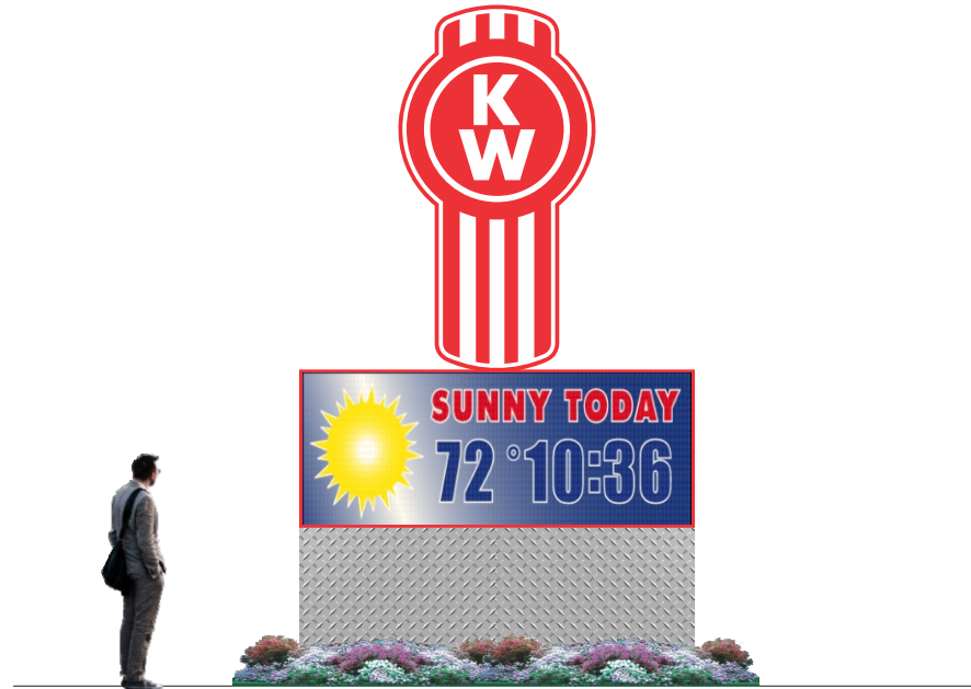
B Front View: Illuminated Cabinet w/ EMC and Diamond Plate Base Scale: 3/16" = 1' - 0"
